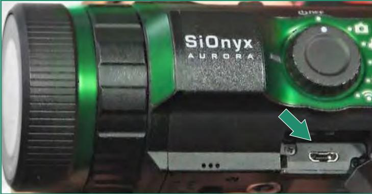
6. Connect the camera to a powered-on computer or plug it into a wall charger using the supplied Micro USB cable.
