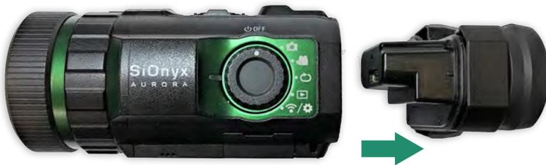
3. Press the tab on the left side of the battery and slide the battery out.
